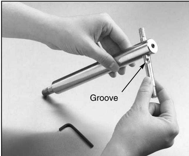
Figure 8. Slide bar into shaft guide.
